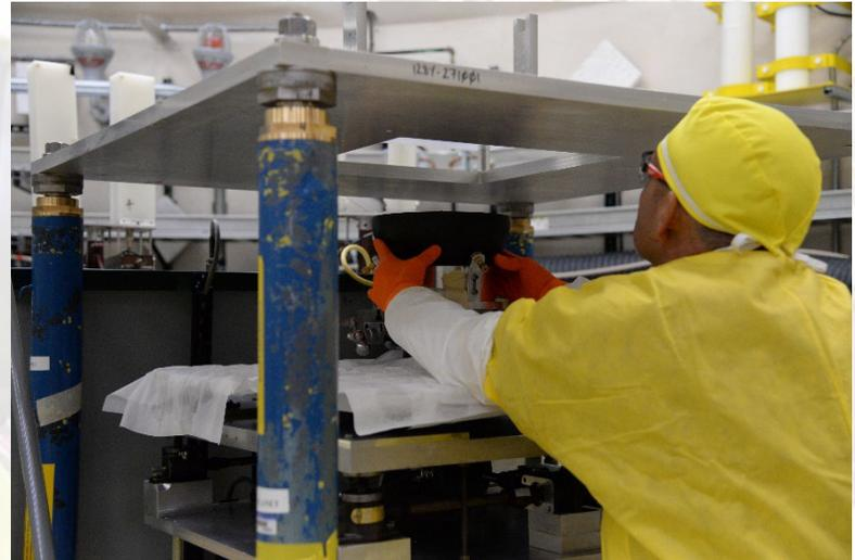
▲ *Kenny Valdez (NEN-2) builds the lower half of the HEU configuration on the Planet moveable platen table. The upper half was later built on the stationary platform.*
