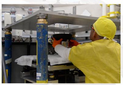
▲ Kenny Valdez (NEN-2) builds the lower half of the HEU configuration on the Planet moveable platen table. The upper half was later built on the stationary platform.
