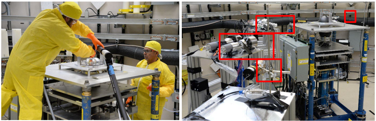
Fig. 2: Left – workers performing Coordinate Measurement Machine (CMM) measurements. Right – organic scintillator measurements of neutron leakage spectra.
