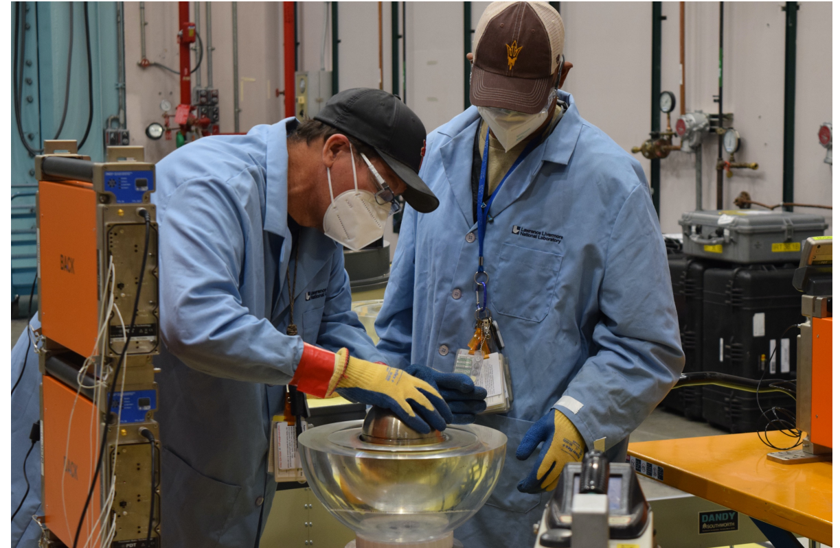
Sealed Radioactive Source encased in steel and plastic
