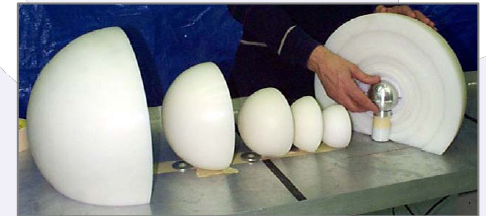
BERP Ball 4.5 kg alpha-phase Pu (94 wt% Pu-239)
