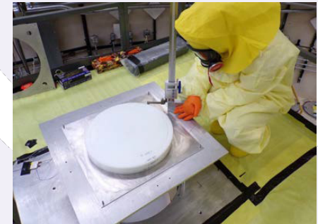
TEX-HEU: Uranium and poly, Hafnium added in next experiment.
