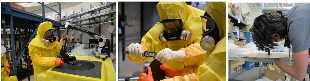
Left: Kristin Stolte measuring one of the Jemima plates with the CMM. Middle: Nicholas Rench measuring the thickness of a Jemima plate with calipers. Right: Zach Lemke measuring the thickness of a copper plate with a micrometer.
