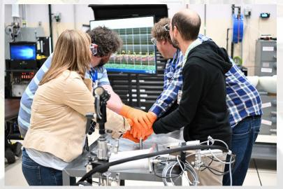
Jesson Hutchinson (NEN-2) demonstrates effects of reflection on system neutron multiplication using a hands-on demonstration with the BeRP Ball.
