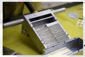
■ ZPPR plates loaded into a 3x2 bucket.
