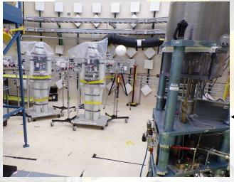
Phantoms and plates positioned in preparation for Godiva burst.
