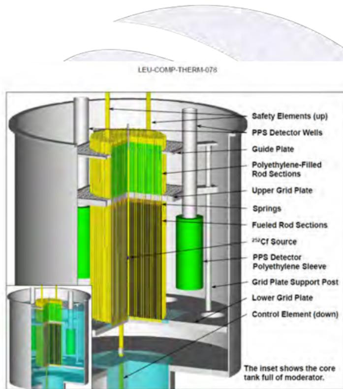
Figure 3. Cut-away View of the Critical Assembly Core Tank (Case 2).
