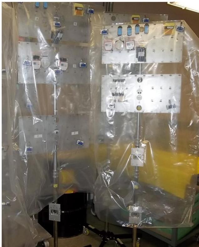
LANL received and positioned the dosimeters in DAF for each of three GODIVA-IV irradiations the week of May 23, 2016. Within hours following an irradiation, the dosimeters were transported to the LLNL NAD Lab for measurement and evaluation. Preliminary dose estimates were collected from each participating laboratory within 24 hours of receipt. Final dose estimates will be completed and published later this year in laboratory reports followed by a summary publication.
