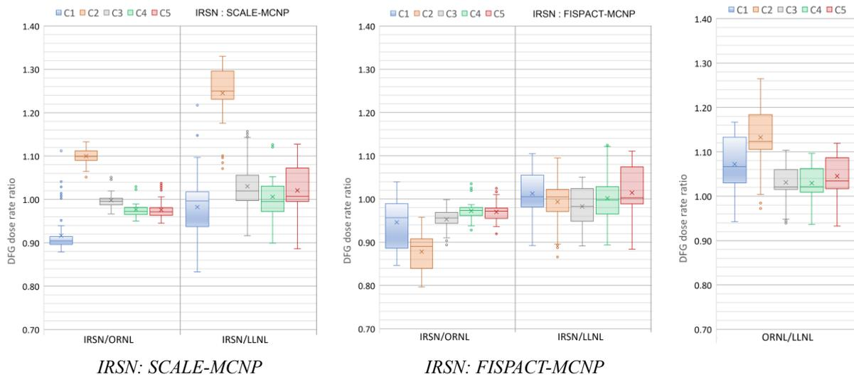
Figure 4. DFG dose rate code-to-code comparison
