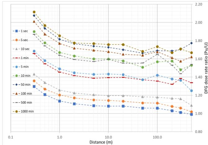
Figure 3. Comparison of DFG dose rates between Pu and U metal
