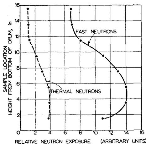
Fig. 8. Relative neutron exposure of samples from side of stainless steel drum.
