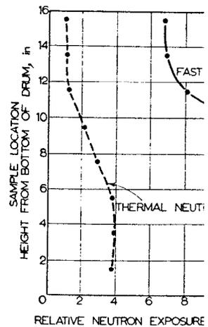
Fig. 8. Relative neutron exposure vs. height from bottom of stainless steel drum.
