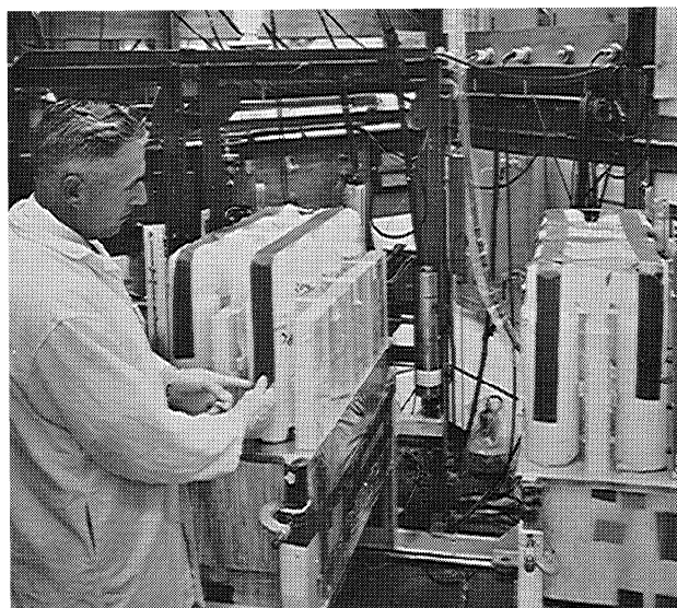
Fig. 1. 16-Bottle moderated unreflected array of ^{233}\text{U} solution.
