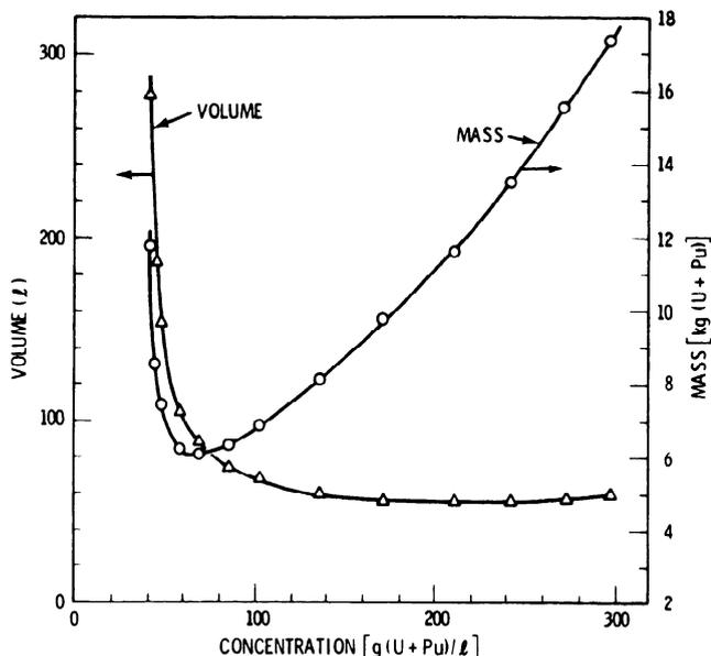
Fig. 2. Criticality of plutonium-uranium solution in cylindrical geometry.
