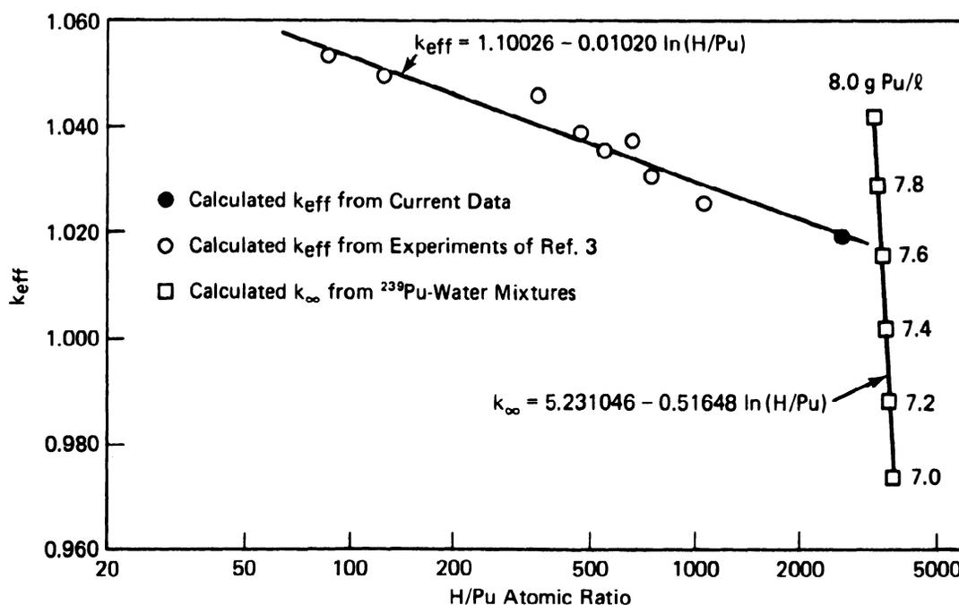
Fig. 2. Experimental eigenvalues and calculated  $^{239}\text{Pu}$ -water data.
