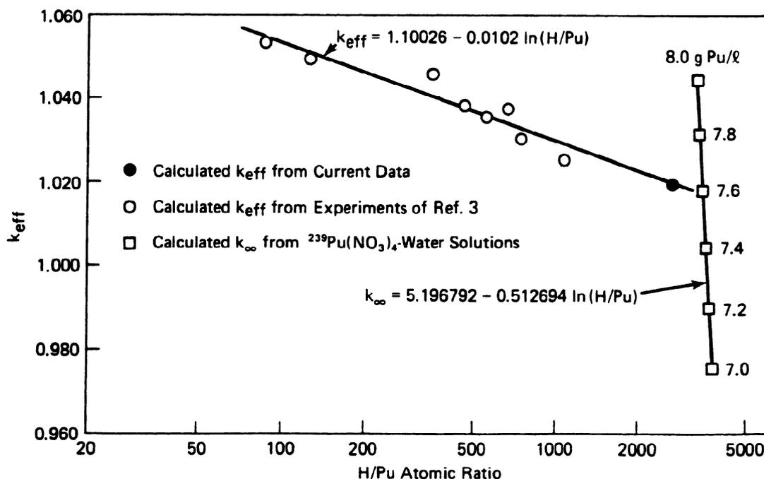
Fig. 3. Experimental eigenvalues and calculated  $^{239}\text{Pu}(\text{NO}_3)_4$  data.
