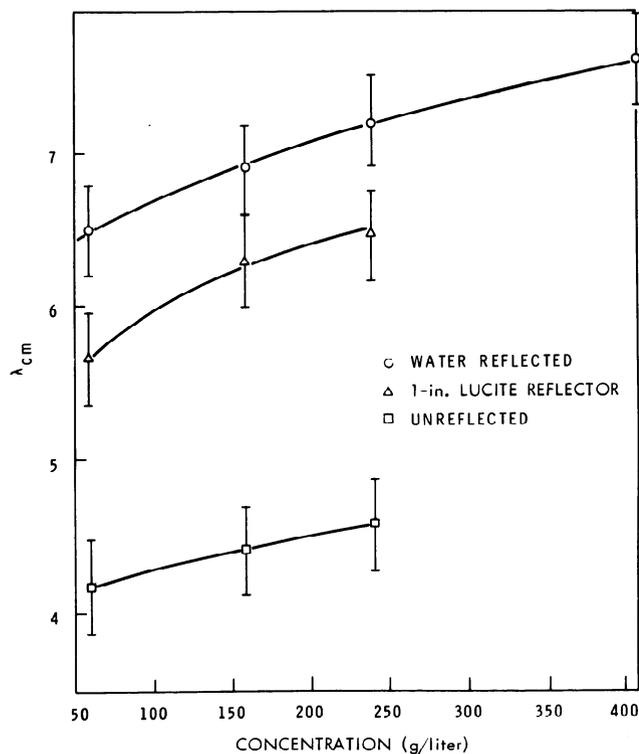
Fig. 2. Extrapolation length—slab tank—18.4%  $^{240}\text{Pu}$ .
