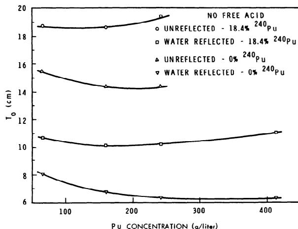
Fig. 3. Effect of  $^{240}\text{Pu}$  on critical slab thickness of  $\text{Pu}(\text{NO}_3)_4$  solution.
