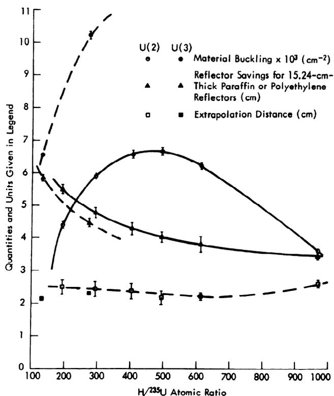
Fig. 2. Material buckling, reflector savings, and extrapolation distance for 2 and 3% <sup>235</sup>U-enriched UF<sub>4</sub>-paraffin mixtures as a function of the H/<sup>235</sup>U atomic ratio.
