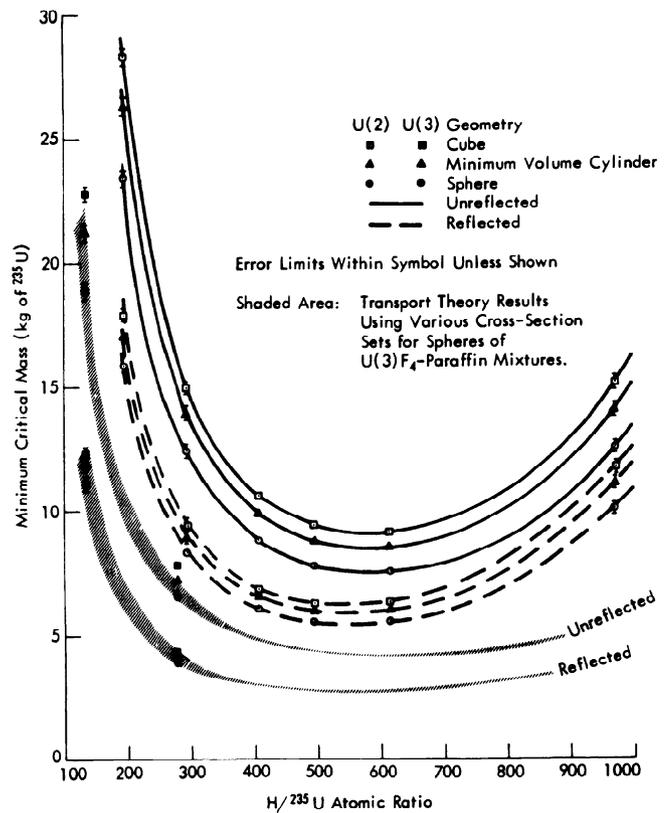
Fig. 4. Critical mass of 2 and 3%  $^{235}\text{U}$ -enriched  $\text{UF}_4$ -paraffin mixtures as a function of the  $H/^{235}\text{U}$  atomic ratio.
