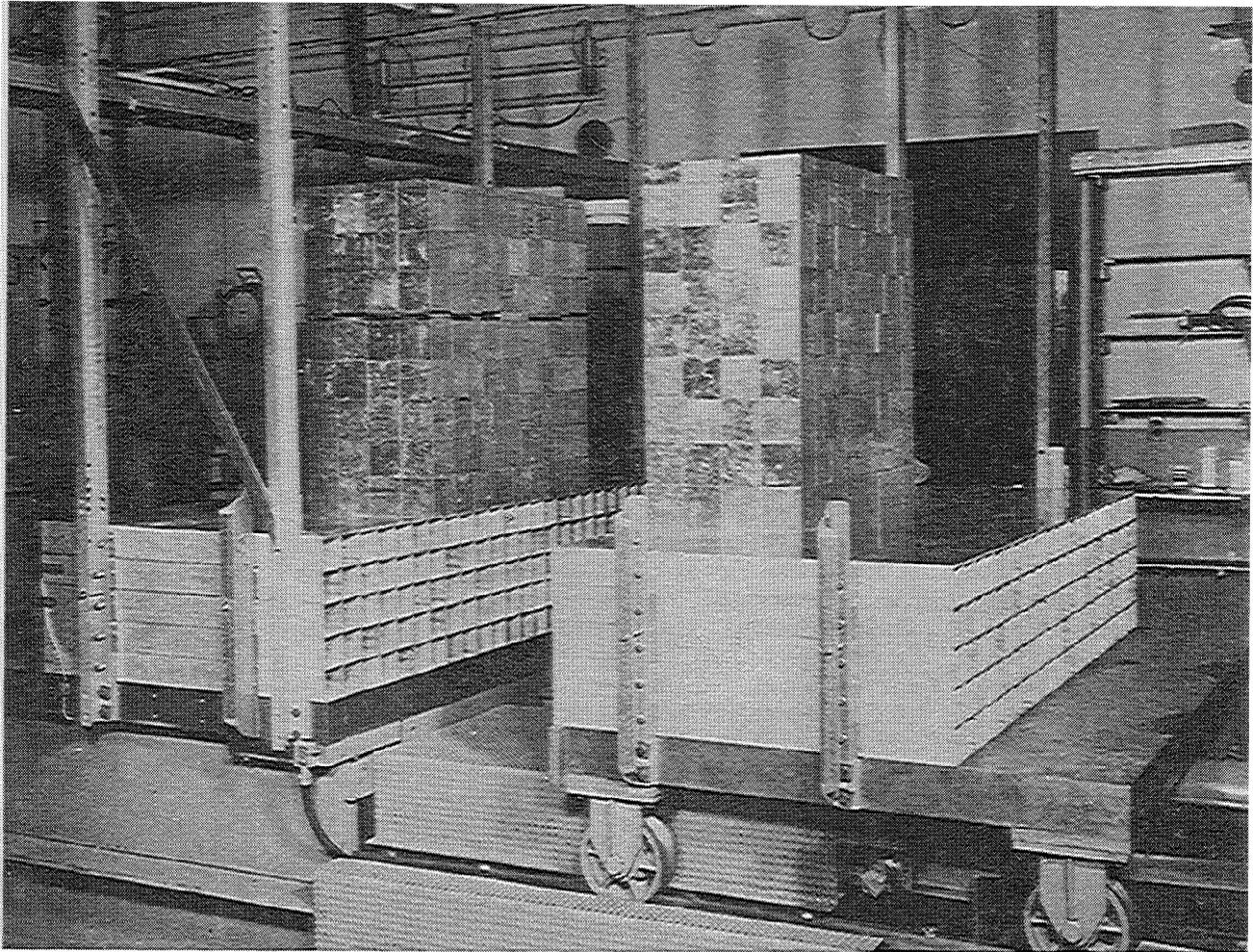
Fig. 1. An experimental assembly on the remotely operated criticality testing equipment.
