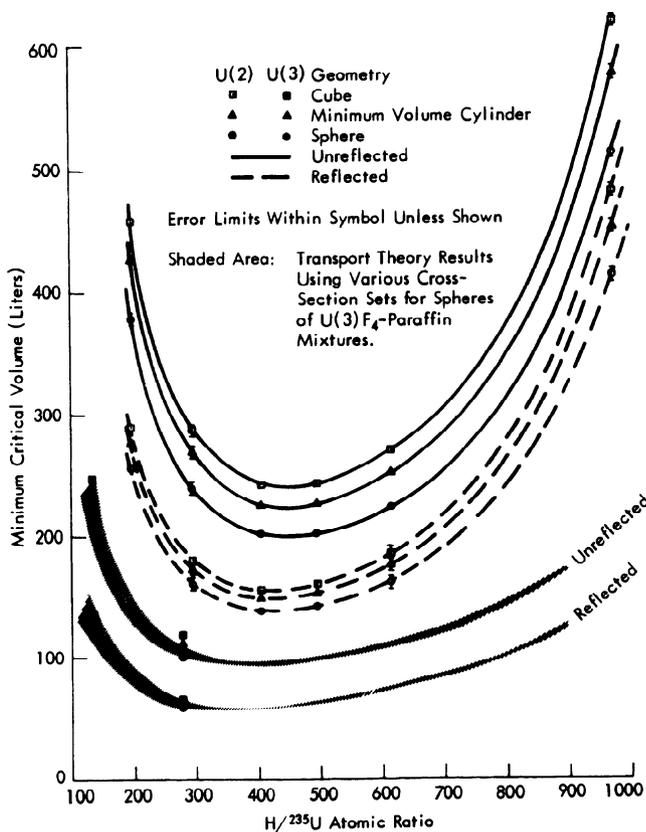
Fig. 3. Critical volume of 2 and 3%  $^{235}\text{U}$ -enriched  $\text{UF}_4$ -paraffin mixtures as a function of the  $H/^{235}\text{U}$  atomic ratio. The values plotted were obtained from experimental data by buckling conversions.
