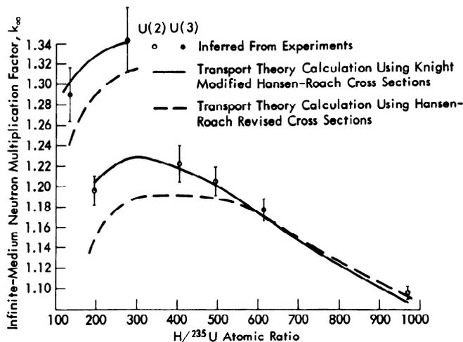
Fig. 7. The infinite-medium neutron multiplication factor of 2 and 3% <sup>235</sup>U-enriched UF<sub>4</sub>-paraffin mixtures as a function of the H/<sup>235</sup>U atomic ratios.
