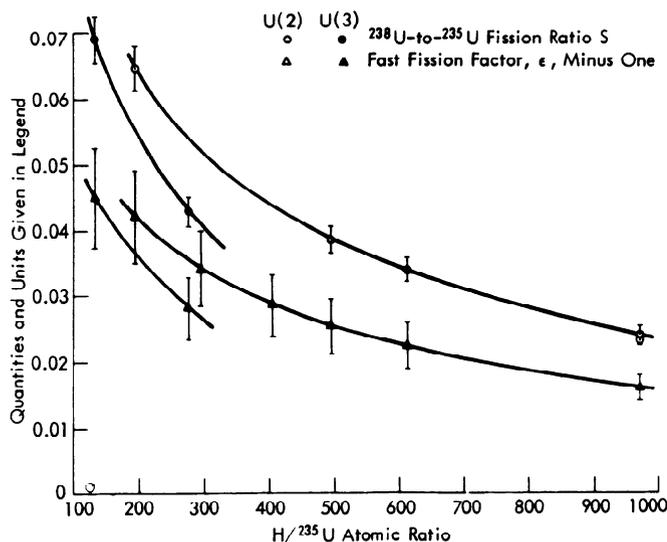
Fig. 6. <sup>238</sup>U-to-<sup>235</sup>U fission ratio and fast fission factor in 2 and 3% <sup>235</sup>U-enriched UF<sub>4</sub>-paraffin mixtures as a function of the H/<sup>235</sup>U atomic ratio.
