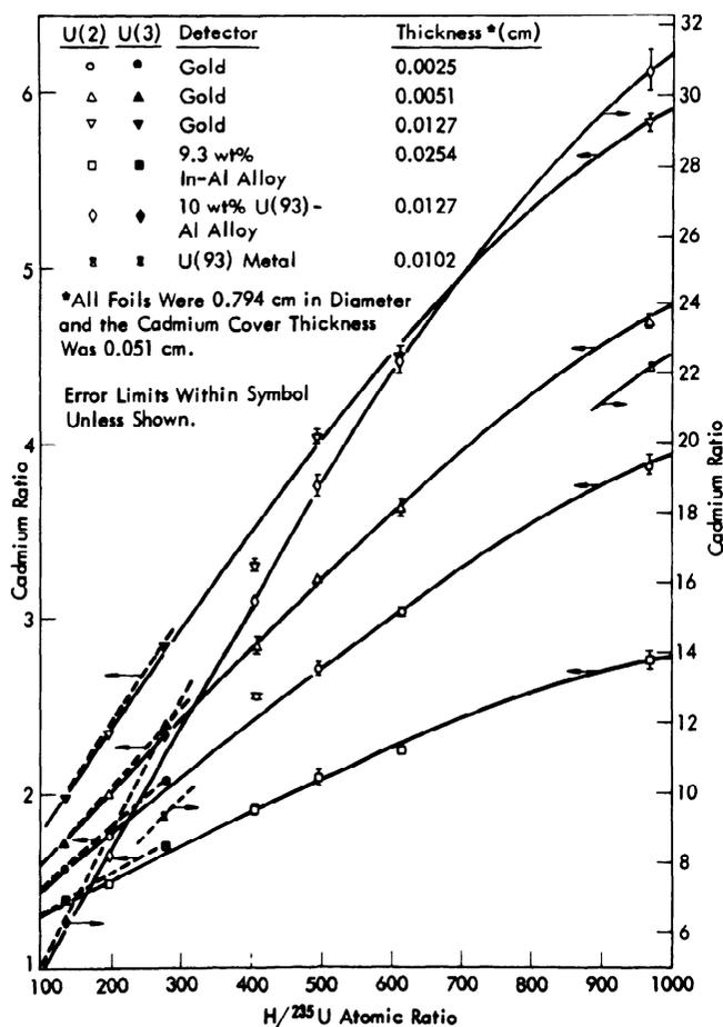
Fig. 5. Cadmium ratios in critical assemblies of UF<sub>4</sub>-paraffin mixtures.
