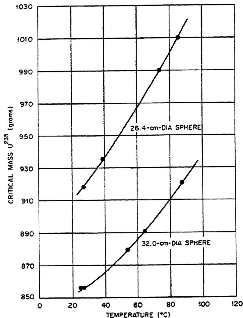
FIG. 5. Critical mass of  $U^{235}$  in water-reflected spherical reactors as a function of temperature.
