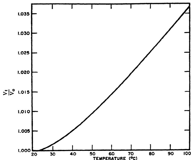
FIG. 1. Volume ratio of  $UO_2F_2$  solutions vs temperature.
