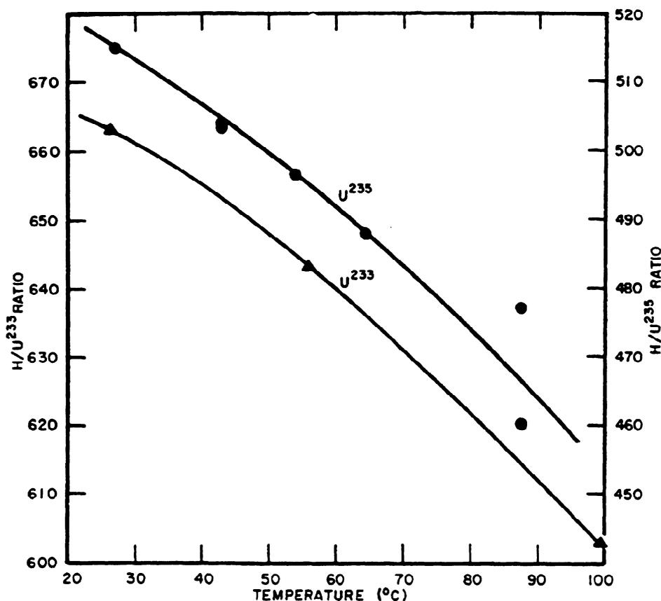
FIG. 4. Ratio of H:U<sup>233</sup> and H:U<sup>235</sup> in 32.0 cm diameter water-reflected spherical reactor vs temperature.
