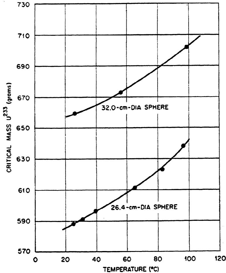
Fig. 6. Critical mass of  $U^{233}$  in water-reflected spherical reactors as a function of temperature.
