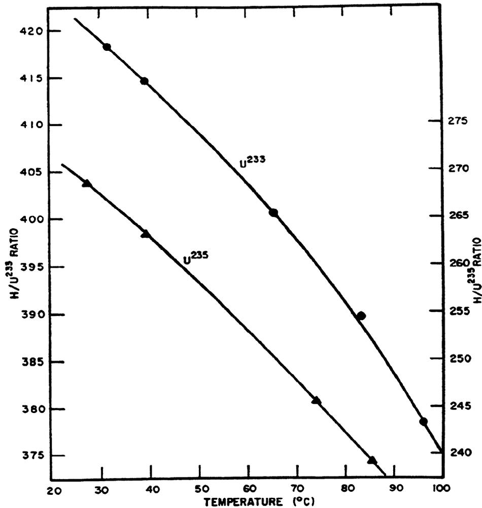
FIG. 3. Ratio of H:U<sup>233</sup> and H:U<sup>235</sup> in 26.4 cm diameter water-reflected spherical reactor vs temperature.
