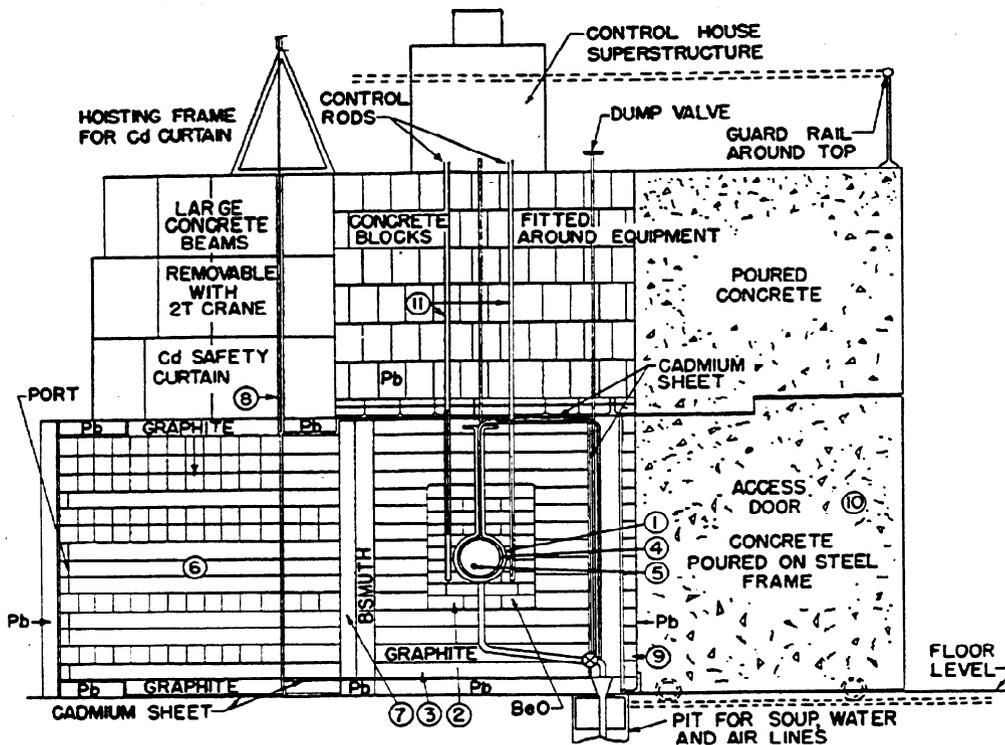
FIG. 4. Section through HYPO (simplified).
