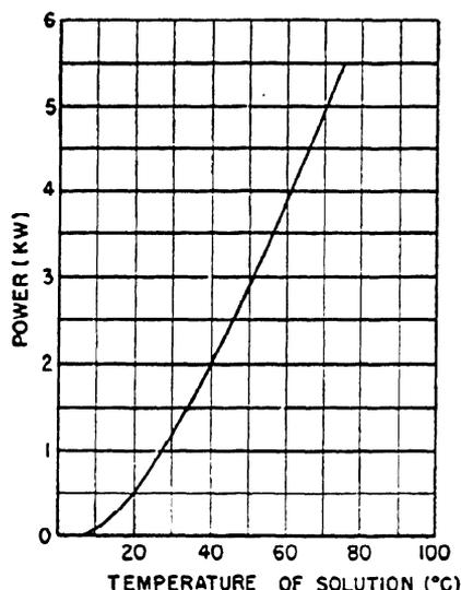
FIG. 8. Equilibrium running conditions for 50 cc/sec inlet water at 8°C.
