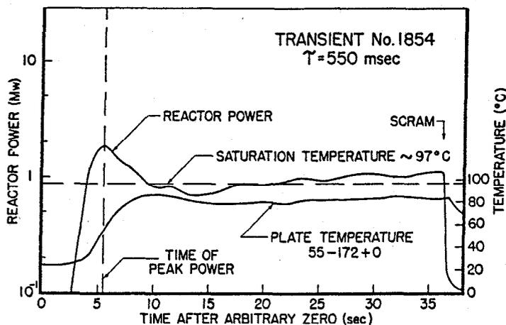
Fig. 5. Representative behavior following 0.60% reactivity addition ( $\alpha = 1.3 \text{ sec}^{-1}$ ).
