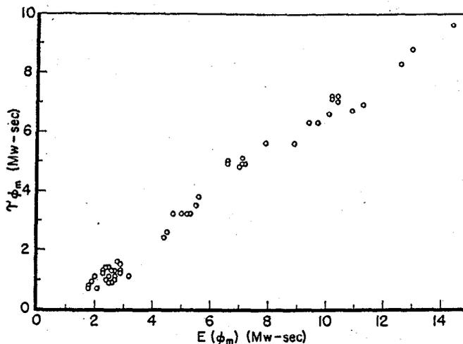
FIG. 14. Product of maximum reactor power  $\phi_m$  and reactor period  $\tau$  versus energy released to time of maximum reactor power  $E(\phi_m)$ .
