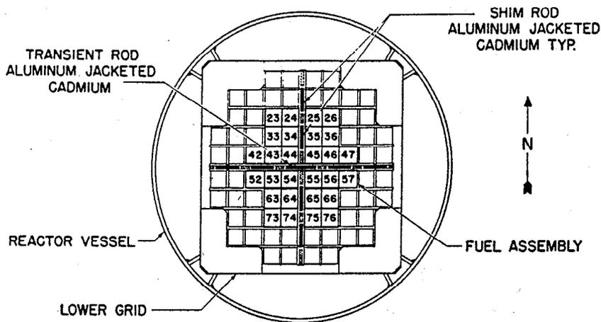
FIG. 1. SPERT I reactor core diagram showing lattice position numbering system.
