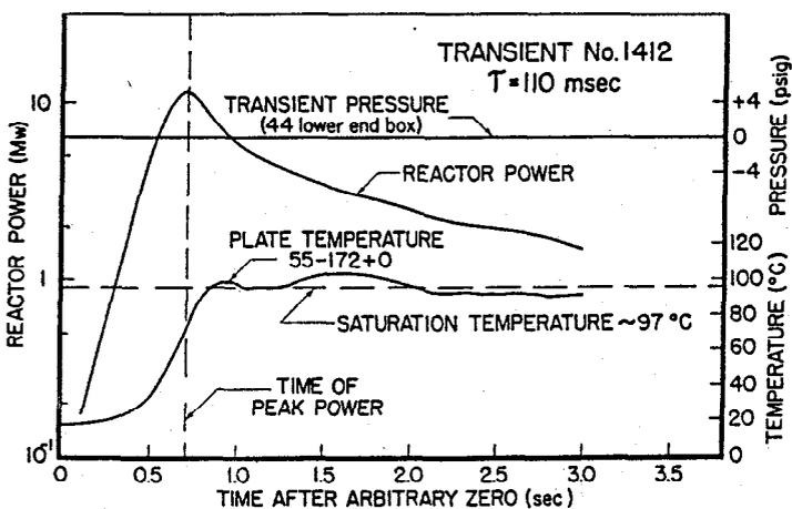
Fig. 6. Representative behavior following 0.71% reactivity addition ( $\alpha = 9.1 \text{ sec}^{-1}$ ).
