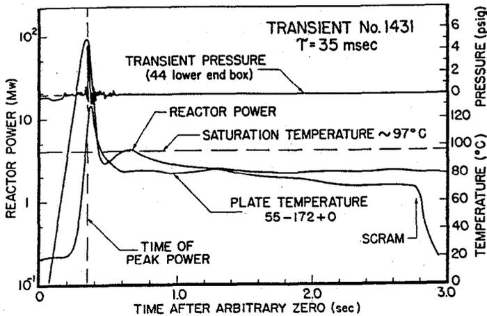
FIG. 7. Representative behavior following 0.85% reactivity addition ( $\alpha = 20 \text{ sec}^{-1}$ ).
