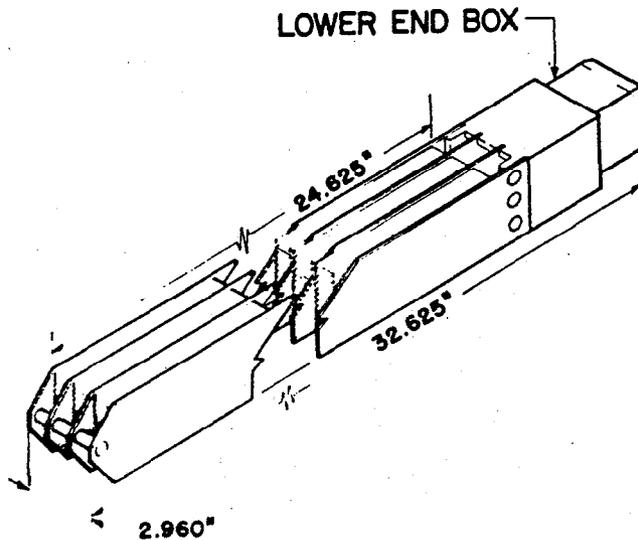
FIG. 2. SPERT I fuel assembly (Type A), showing fuel plate numbering system. Location of thermocouples is specified by three coordinates: (1) lattice position (see Fig. 1), (2) fuel plate number, (3) distance from horizontal center line of reactor core in inches (positive up). For example, 55-172-3 indicates a position 3 inches below centerline on the south center plate of the assembly in position 55.
