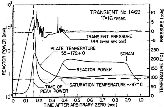
FIG. 8. Representative behavior following 1.0% reactivity addition ( $\alpha = 62 \text{ sec}^{-1}$ ).
