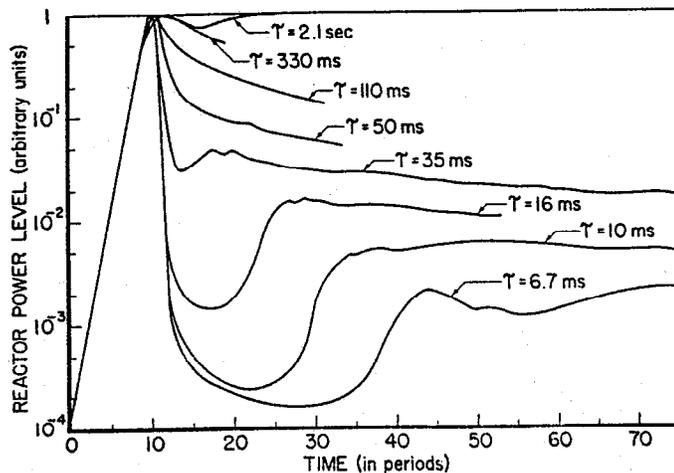
FIG. 10. Power burst shape as a function of initial reactor period  $\tau$ . Power curves have been normalized at peak values and are plotted in units of  $\tau$ .
