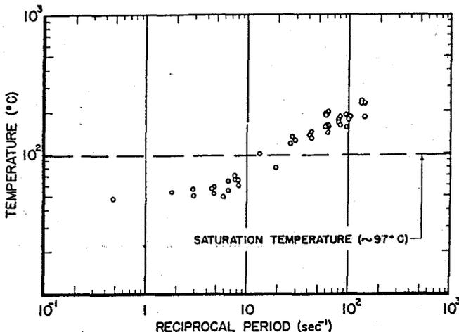
FIG. 16. Fuel plate surface temperature at the time of maximum reactor power as a function of reciprocal reactor period. Thermocouples were located at horizontal center line of reactor core in a central fuel assembly.
