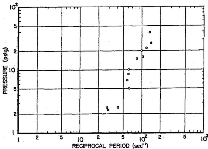
FIG. 17. Maximum transient pressure as a function of reciprocal reactor period. Pressure transducer was located in lower endbox of a central fuel assembly.
