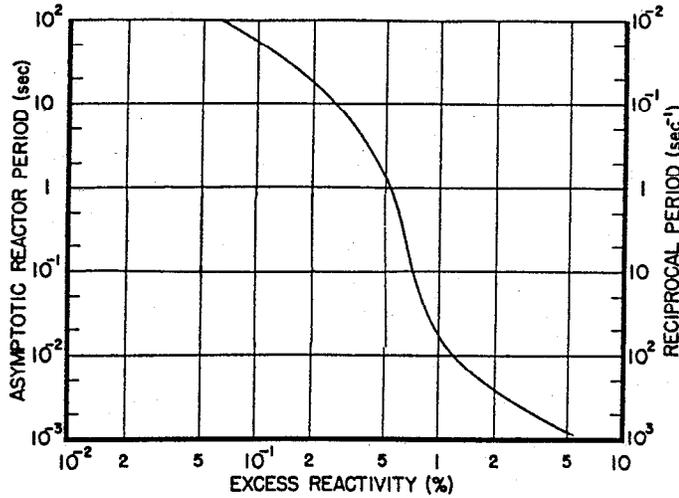
FIG. 3. Excess reactivity versus asymptotic reactor period (in-hour relation) for effective neutron lifetime of 50  $\mu$ sec using Keepin and Wimmatt delayed neutron data (7).
