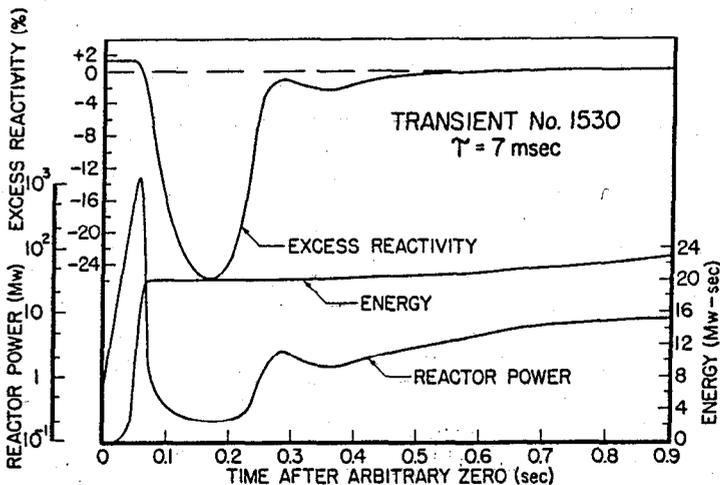
Fig. 20. Instantaneous excess reactivity during a 7-msec period transient test. Also shown are reactor power and energy release.
