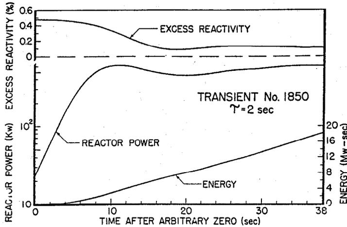
FIG. 18. Instantaneous excess reactivity during a 2-sec period transient test. Also shown are reactor power and energy release.
