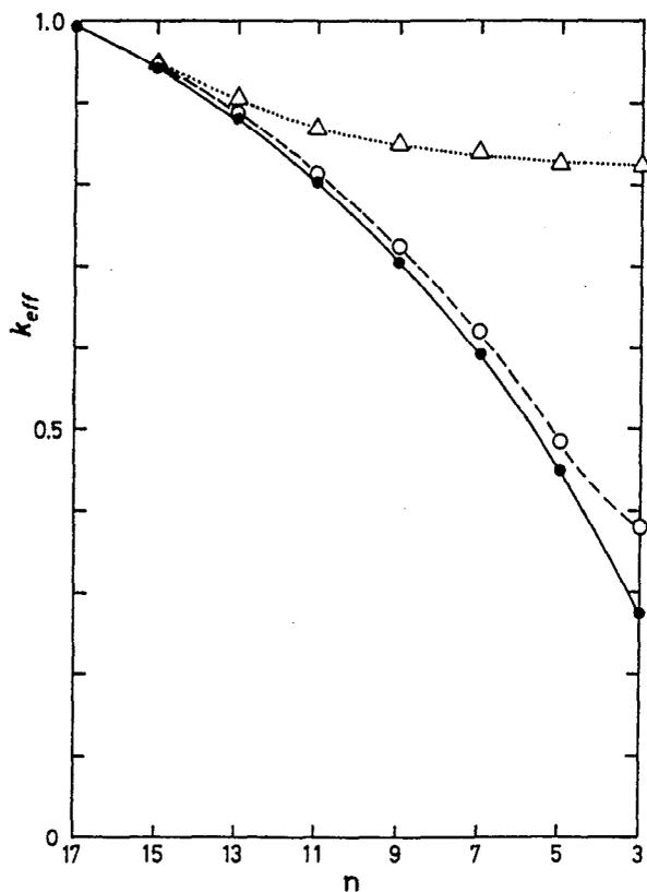
Fig. 2. Comparison among experimental and calculational effective multiplication factors  $k_{\text{eff}}$ . Closed circles, open circles, and triangles represent KENO IV, exponential, and pulsed-neutron source results, respectively.  $N$  is of  $n \times n$  square lattices.
