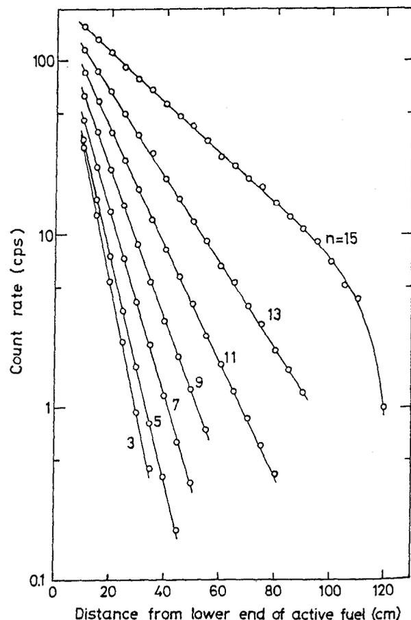
Fig. 1. Vertical flux distribution obtained by exponential experiment.
