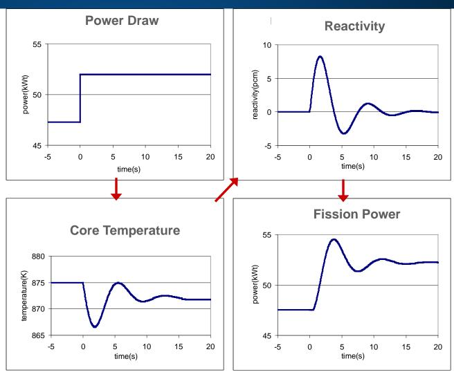
Note: this reactor has 2 components, core and reflector. In this scenario, the increased power causes an increase in reflector temperature, which creates a small net reactivity drop, thus the core settles at a lower temperature to compensate.
