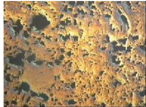
Nuclear Graphite (SEM at NCSU) Density = 1.5 - 1.8 \text{ g/cm}^3
