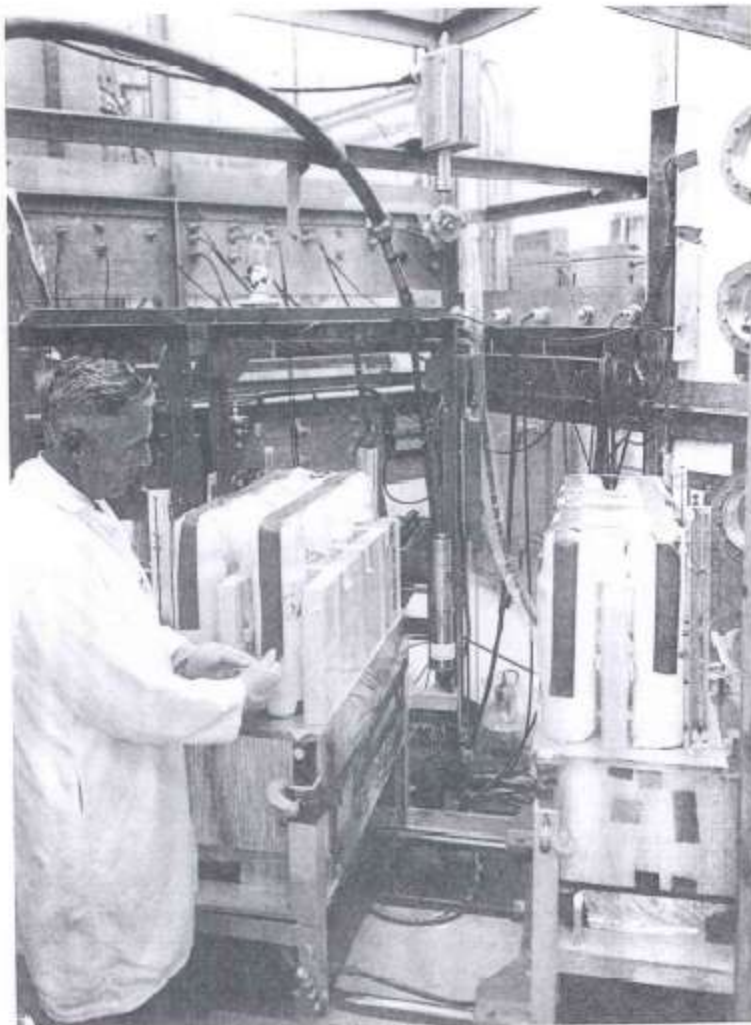
Figure 30. Criticality of Arrays of ^{235}\text{U} Solution (16-Bottle Moderated Unreflected Array of ^{235}\text{U} Solution) 50
