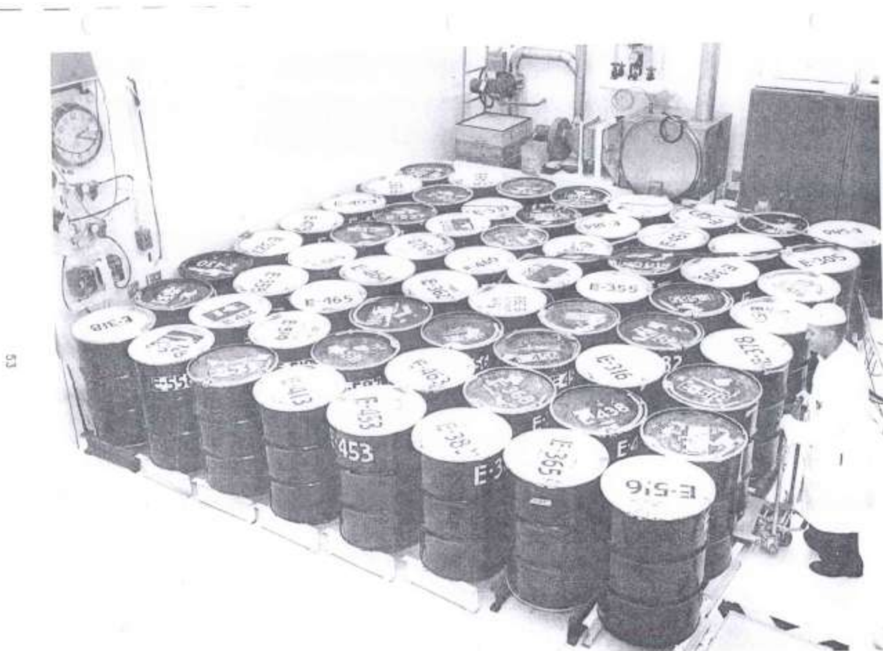
Figure 32. Subcritical Neutron Multiplication Measurements on Arrays of Storage Containers for Plutonium Nitrate Solution
