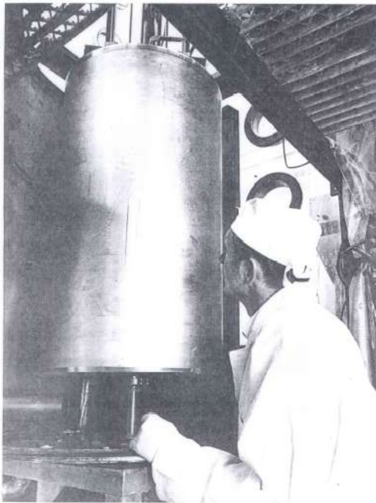
Figure 17. Cylindrical Vessel Being Set Up for Criticality Studies with Solutions
