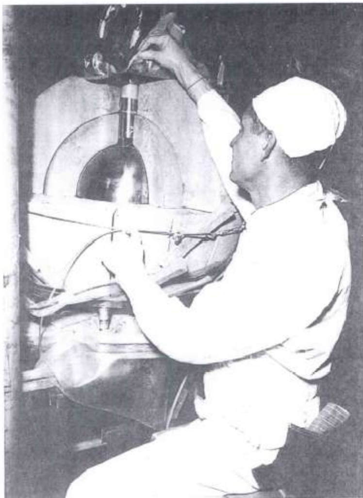
Figure 13. Vessel for Studying Criticality of Solutions in Spherical Geometry with Concrete Reflector Partially Removed
