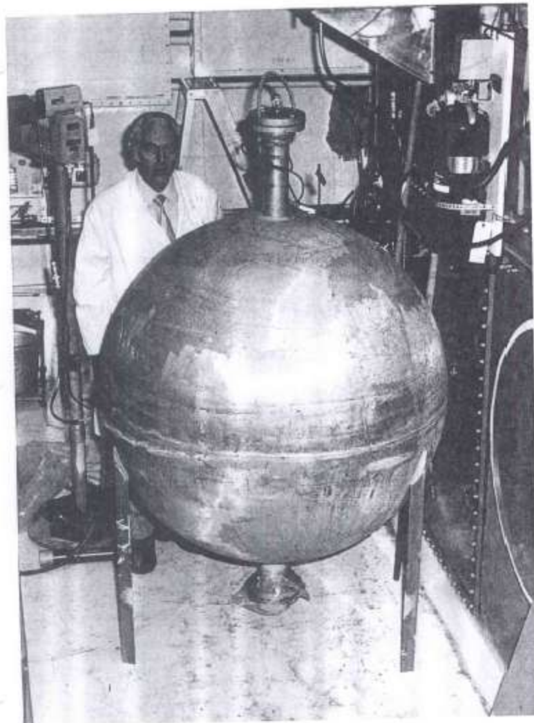
Figure 16. Large Spherical Vessel Used for Determining Eta for Plutonium and Infinite Sea Critical Concentration
