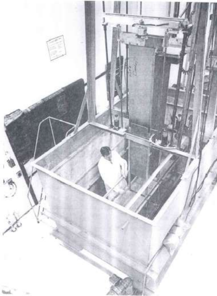
Figure 8. Facility for Studying Criticality of Arrays of Fuel Elements in Water
