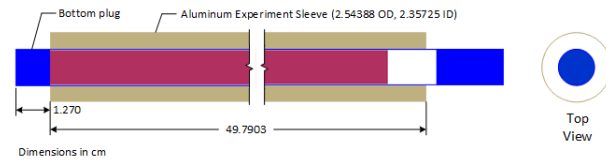
Fuel Element with Aluminum Sleeve
