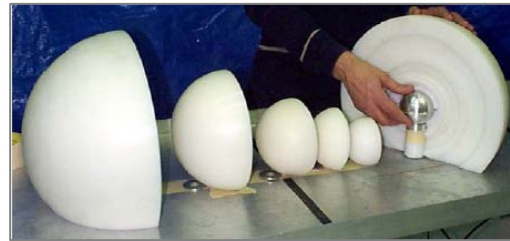
BERP Ball 4.5 kg alpha-phase Pu (94 wt% Pu-239)
